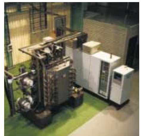
Laser-Arco ® - the technology to deposit Diamor ®
