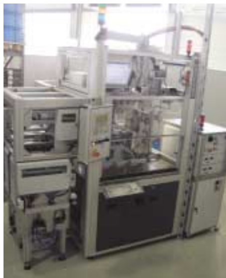
Laser hardening system at Sitec Industrietechnologie Chemnitz
