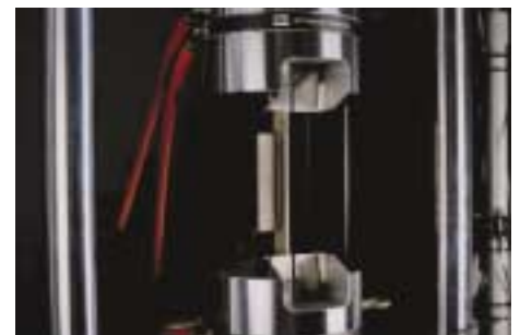
Servo hydraulic fatigue testing of laser hybrid welding joints for steel based lightweight constructions
