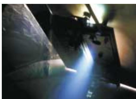
Arc coating of temperature sensitive fibers
