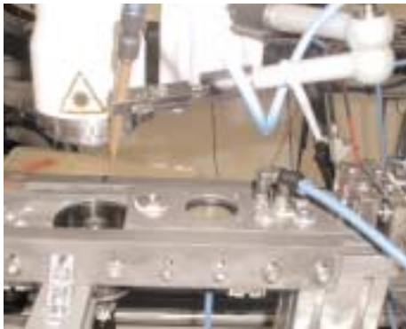
Development of a laser hardening process under protective gas for injection system parts
