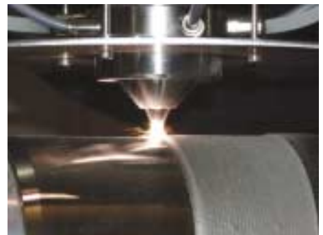
Laser powder deposition welding of the wear ring of an industrial oil drill tool
