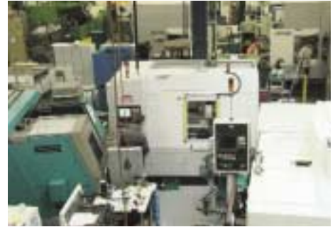
Laser hardening system in series production at BorgWarner in Kirchheimbolanden (system integrator EFD)
