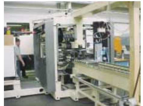
System for the induction assisted laser welding of automotive drive shafts at Visteon in Dueren (system integrators Arnold and EMAG)
