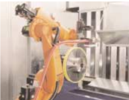
Atmospheric plasma spraying with laser coupling
