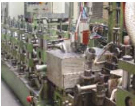
System to weld high-quality steel pipes at Abrecht Zwick GmbH, Hagen
