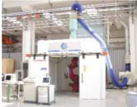
Remote laser welding system at Salvagnini (Italy)
