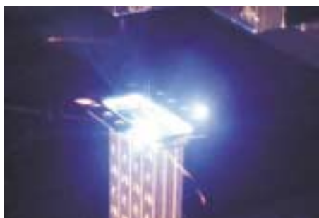
Welding of the tube / base plate joint of an exhaust gas heat exchanger utilizing a beam scanning optics
