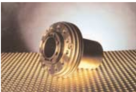
Part of the main drive shaft of a lathe, which was hardened with a high power diode laser
