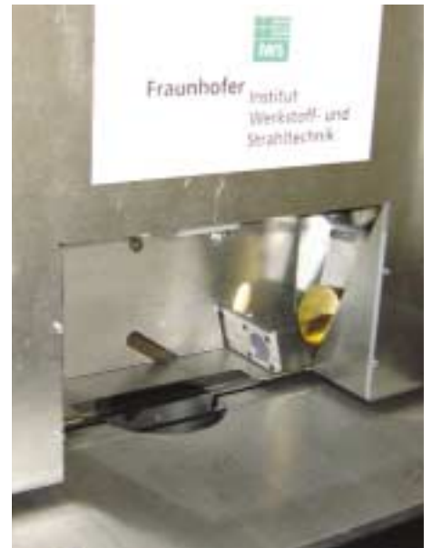
New measuring device for FTIR quality control of wafers
