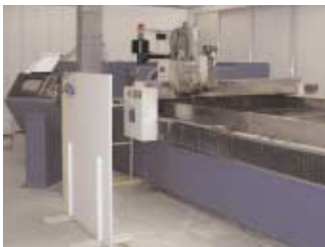
Beam technology: Water jet abrasive cutting machine
