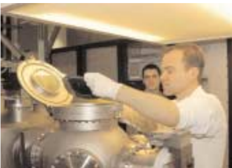
Substrate loading at an EUV precision coating machine for the manufacturing of nm-multilayer coatings
