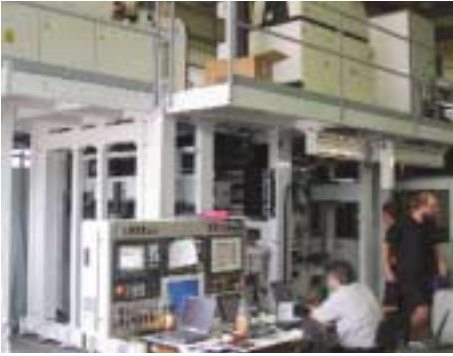
Laser welding system for the joining of differential transmissions (system integrator Arnold)
